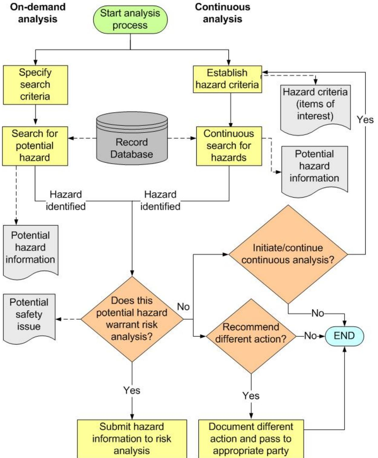
Figure 3: Hazard Identification in On-Demand and Continuous Analysis
