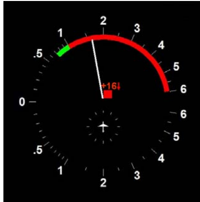
Adjust Vertical Speed as shown on IVSI and EFIS displays (in this example reduction to 1000 ft/min against a threat above)
