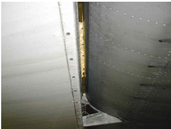
Frozen residues between elevator and horizontal stabilizer on a BAe 146
