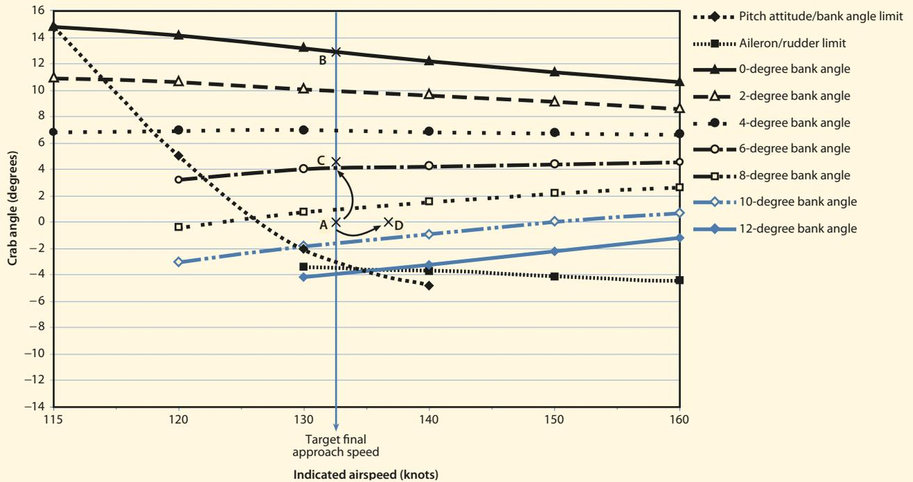
**Examples:** A sideslip landing (zero crab angle) requires about a nine-degree bank angle at touchdown (point A). A wings-level landing (no decrab) requires about a 13-degree crab angle at touchdown (point B). Point C represents a touchdown using a combination of sideslip and crab angle (about five degrees of bank angle and about five degrees of crab angle). Point D represents a steady-sideslip landing conducted about four knots above  $V_{REF}$ .
