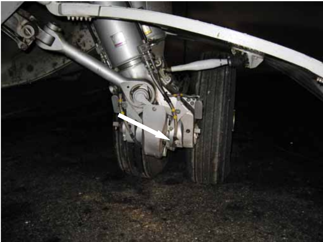
Figure 2. The damage detected on the left main landing gear. The arrow points the damaged anti skid wiring.
