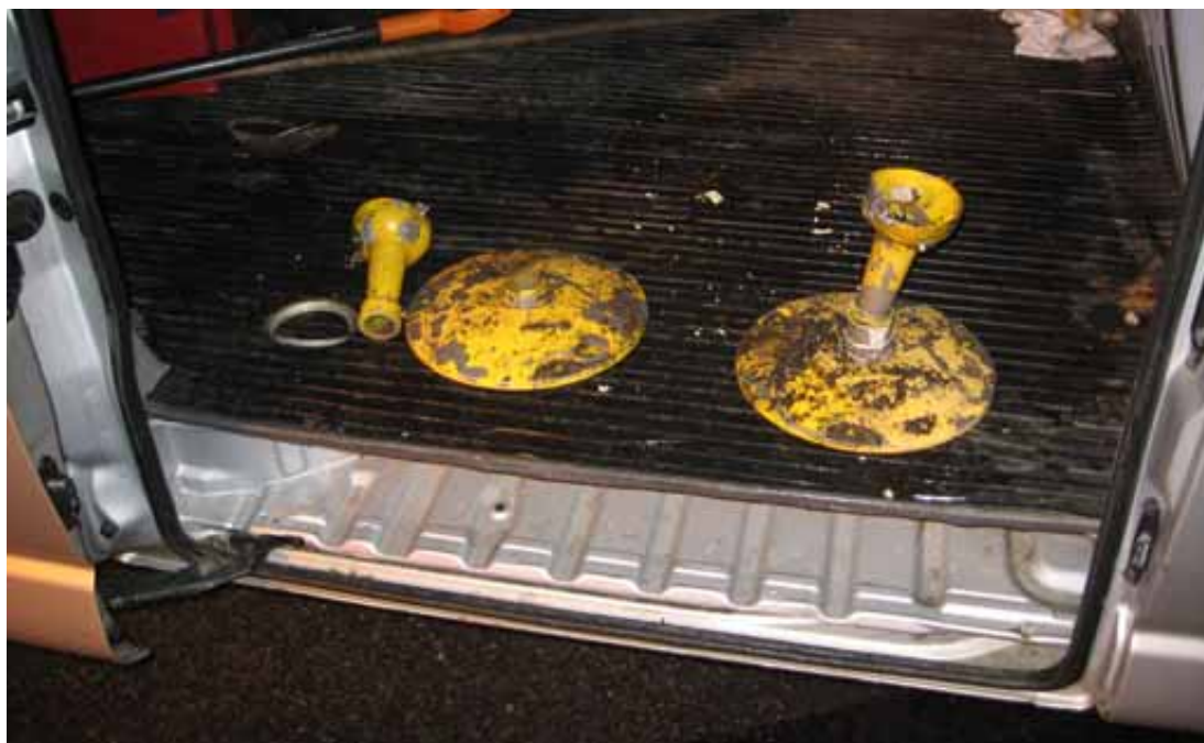
Figure 1. Broken runway edge lights
