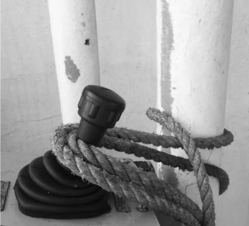
Figure 1: Winch control lever tied with a rope
