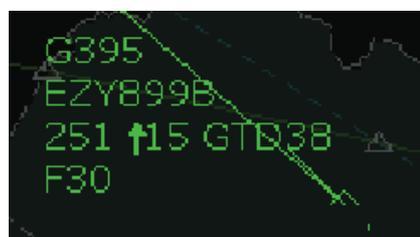
Flight EZY 899B is in contact with a sector below sector L5. It is cleared to climb to flight level FL 300 (F30).
