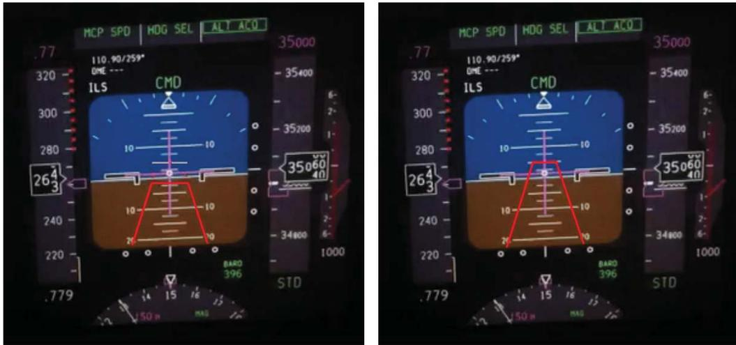
**Figure 14:** Preventive resolution advisory “MONITOR VERTICAL SPEED” on the left and corrective advisory “CLIMB, CLIMB” on the right
