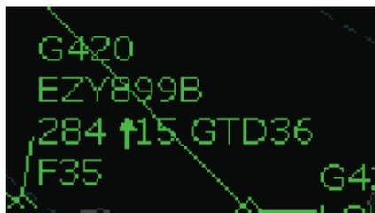
Flight EZY 899B is in contact with a sector below sector L5. It is cleared to climb to flight level FL 350 and the value of its assigned cruising level is now FL 360.
