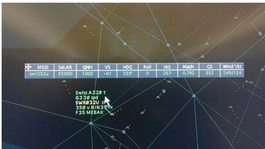
**Figure 5:** Example of the MSID window display
