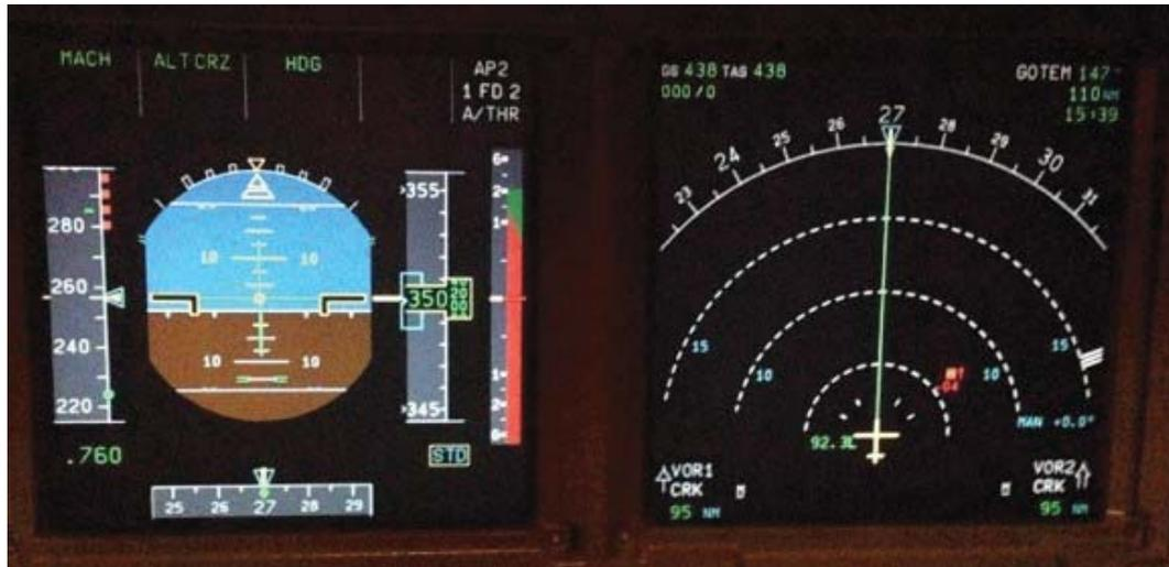
**Figure 6:** Visualization of a “CLIMB” resolution advisory on the PFD and ND of the A320 in the left-hand position
