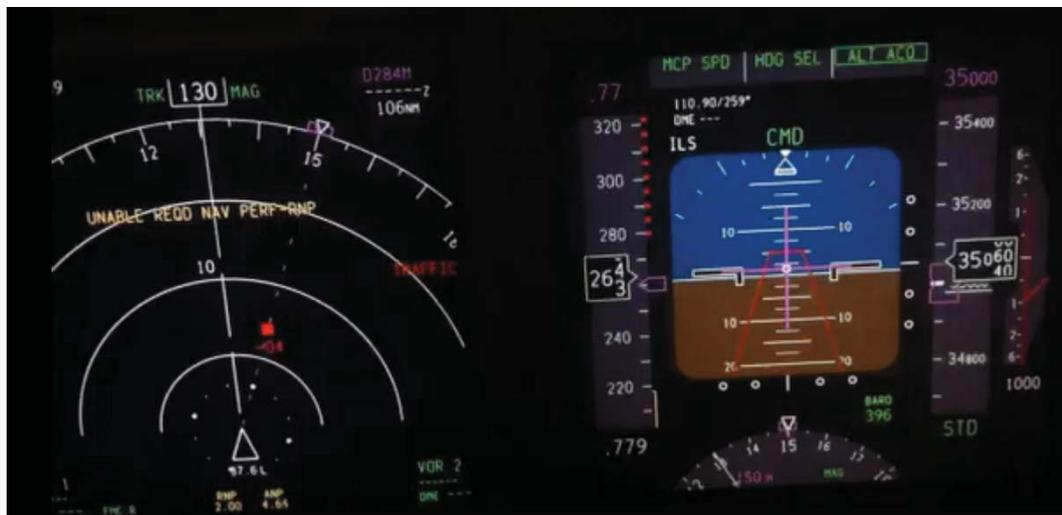
**Figure 7:** Visualisation in the right-hand position of a “CLIMB” on the PFDs and NDs of the Boeing 737-800
