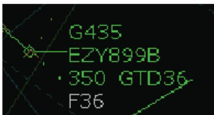
Flight EZY 899B is in contact with sector L5. It has received clearance to climb to flight level FL 360 (F36). The “close the loop” manipulation by the RP controller has not yet been carried out (F36 in white). When it has been carried out, “F36” will change to green.
