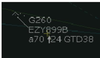
The label of flight EZY 899B after correlation. ATM links the data from the flight plan and the information transmitted by the aircraft's transponder. Its current altitude is 7000 ft (a70) and ATM assigns it the requested cruising level, FL 380 (38).
