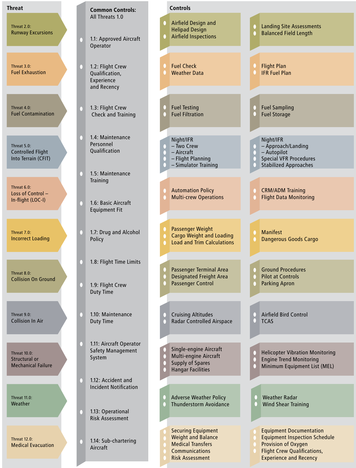
Figure 1: BARS Bow Tie Risk Model – Schematic of Aviation Risk Management Controls and
