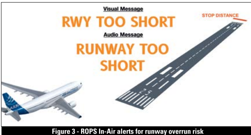
Figure 3 - ROPS In-Air alerts for runway overrun risk
