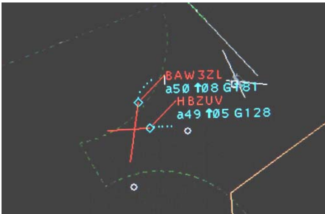
Figure 4: Representation of the situation just before the point of closest approach of the two aircraft according to the legal recording. The above picture serves as illustration of the STCA alert who also was displayed in aerodrome control. The red flight plan call signs and the red directions of movement show the STCA warnings and indicate an impending conflict.
