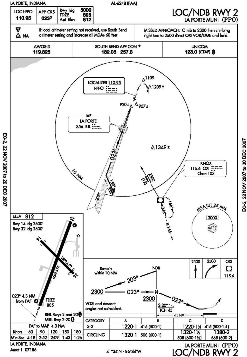
**FIGURE 5. INSTRUMENT APPROACH PROCEDURES WITH CONTROLLING STEPDOWN FIX**
