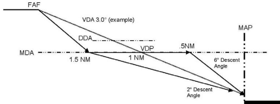
In this example, the aircraft leveled at the MDA (dive and drive) and is proceeding to the MAP in an attempt to acquire the required visual references to continue the approach below the MDA. The 3.0° VDA would be used in this example to fly a CDFA.
