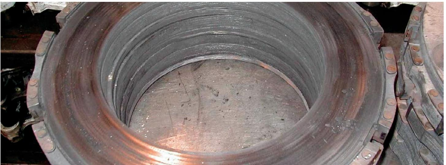
**Figure 4: Catalytically oxidized carbon pressure plate disk failure resulting in a brake fire after landing**
