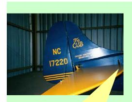
4. Trimming tailplanes aren't confined to the jets – this Piper Cub has one, as shown by the slot near the tailplane l.e. which provides access to the actuating link
