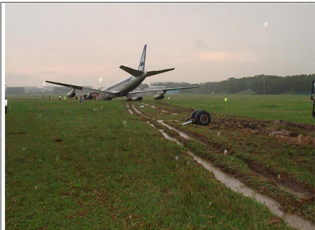
On 13 December 2002, a McDonnell Douglas DC-8-62 freighter overran Runway 20R while landing at Singapore Changi Airport. The overrun occurred after the aircraft landed long (by about 1,300 metres) on the runway in heavy rain. The aircraft sustained substantial damage during the overrun. None of the four persons on board was injured.
