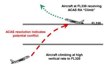
Logic modifications mean that the majority of RAs issued in these situations do not now require a move off level by the level aircraft, or a reversed vertical rate by the climbing/descending aircraft. However, occurrences of RAs can be minimised if pilots adjust their rate of climb/descent to 1500 ft per min. when they are approaching an altitude 1000 ft above, or below, their cleared level.
