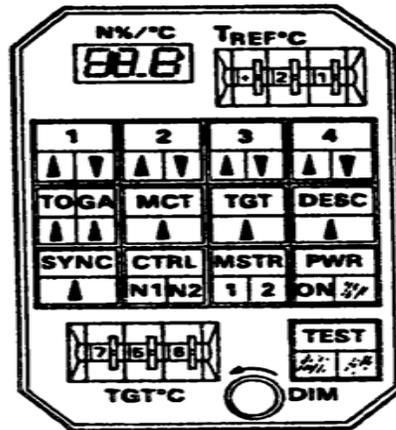
Figure 5: Control Display Unit (CDU)
