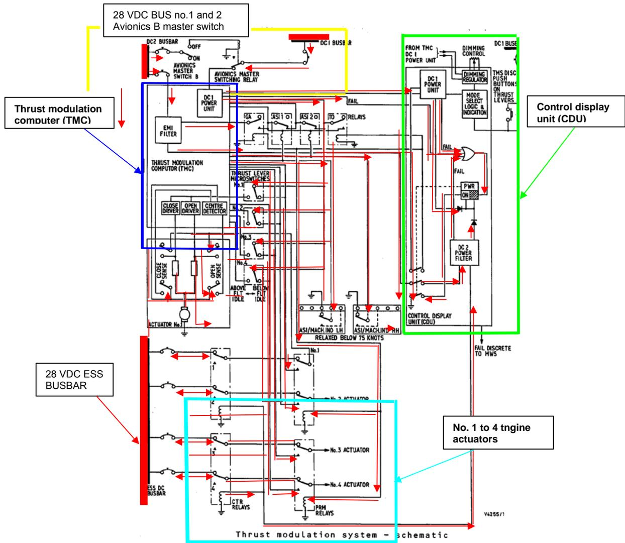
Figure 4: Wiring diagram of the TMS
