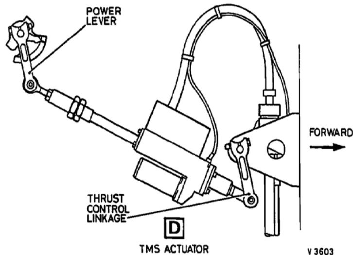
**Figure 6:** Throttle modulation system actuator
