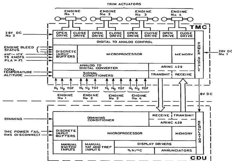
Figure 7: Block diagram of TMS
