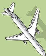
Pilot initiates slideslip. Left rudder pedal pushed while he turns the yoke to the right. Aircraft manoeuvred into a steep angle. Aircraft rapidly loses altitude.
