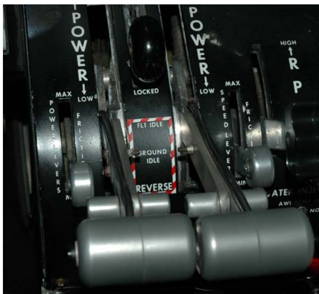
Figure 1: Power levers and markings
