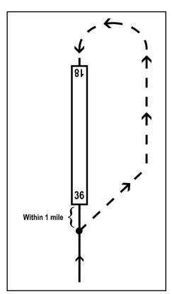
Figure 2. "Classic" circle-to-land scenario with electronic guidance to Runway 36, followed by circling maneuver to Runway 18. In this situation, don't depart the electronic final approach guidance until within one mile of the approach end of the runway served by the IAP.
